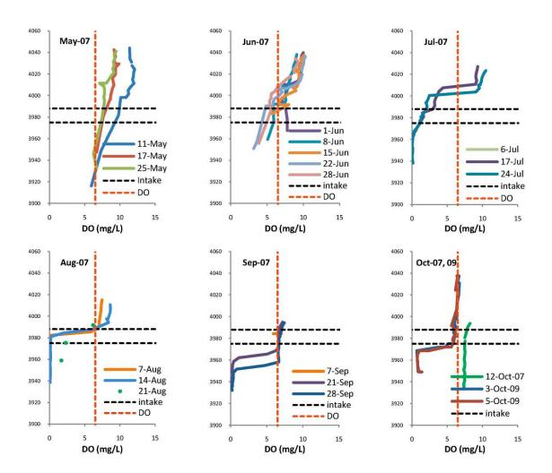
Figure 5-3 Phillips Lake Dissolved Oxygen Profiles Based on Data Collected Between May and October 2007 and October 2009
