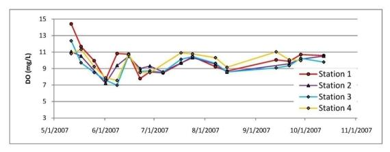
FIGURE 9: 2007 DISSOLVED OXYGEN DATA IN % SATURATION FOR THE POWDER RIVER
